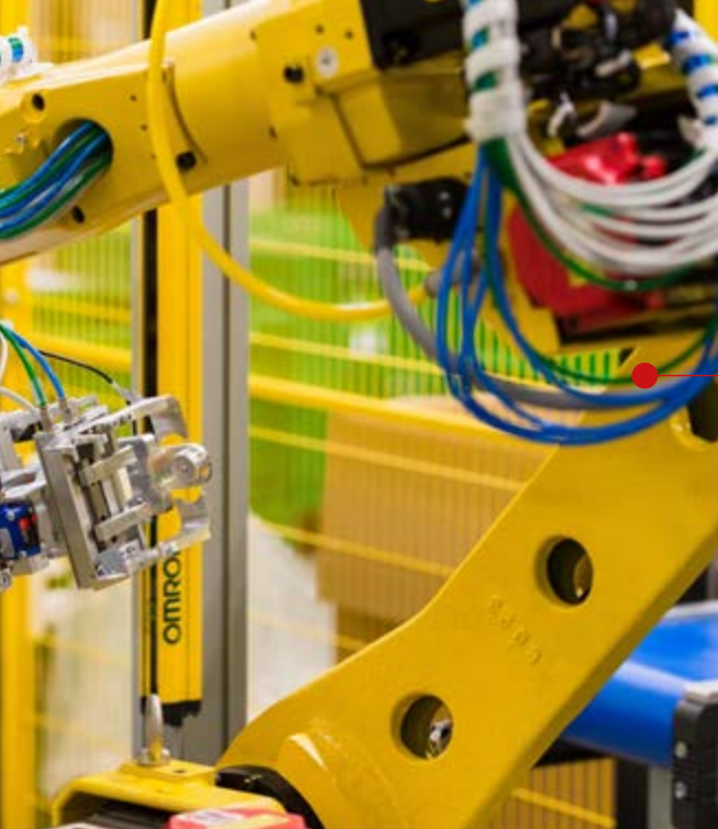
Collection of tank semi-shells by anthropomorphic robot
